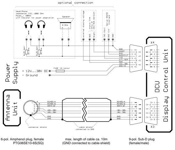
Fig. 2-6 Interwiring Diagram
