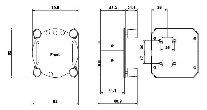
Fig 2-1 Dimension Drawing of the Display Unit
