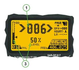
Fig. 3-6 Display Page 3 (Bearing Display as Text)
