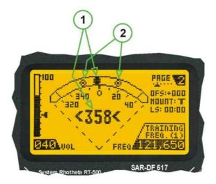
Fig. 3-5 Display Page 2 (expanded +/- 45° Bearing Display)
