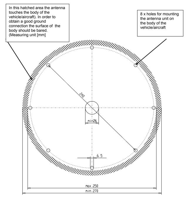
Fig 2-3 Mounting Drawing of the Antenna
