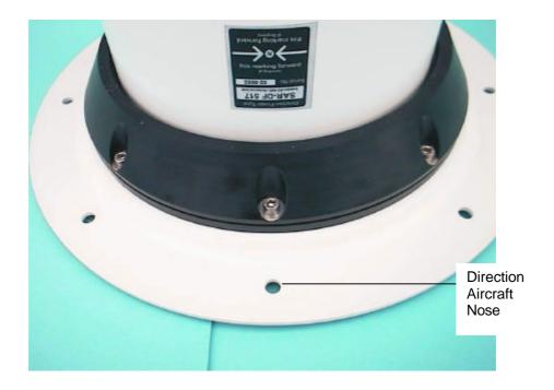
Fig. 2-5 Montage direction of the antenna unit
