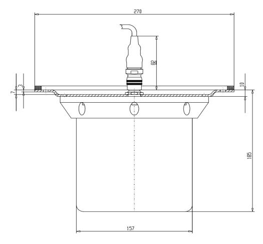
Fig 2-4 Dimension Drawing of the Antenna
